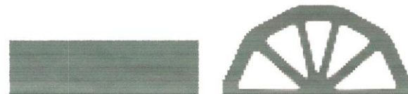
Figure 7.2: Optimal bridge in 2 d: half domain initialization and optimal shape after 100 iterations.
