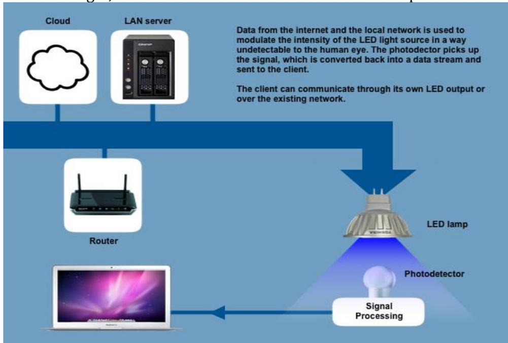
Figure 1: Li-Fi (Light Fidelity): The Future Technology in Wireless Communication 1689
