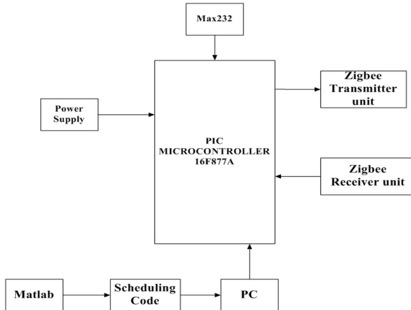
Figure 3.1: Base station Block Diagram
