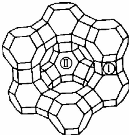
**Figure 7: Zeolite X structure**
