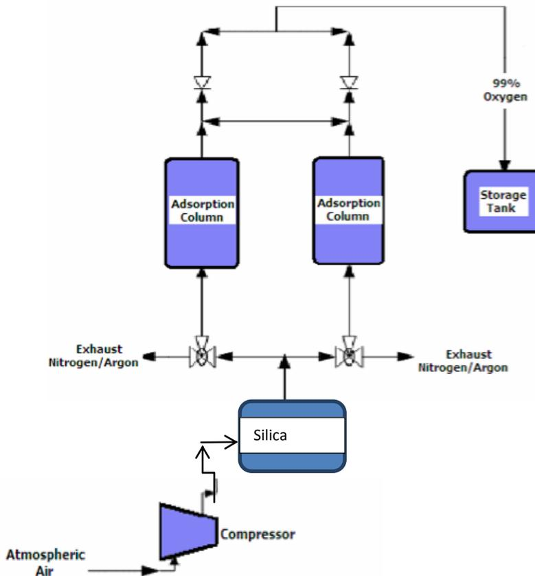
**Figure 9: PSA Process Flow Diagram**
